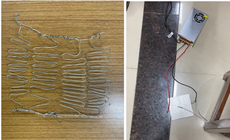
Figure 34: The nichrome wire layout(left) and the final heating module with mica sheets(right)
