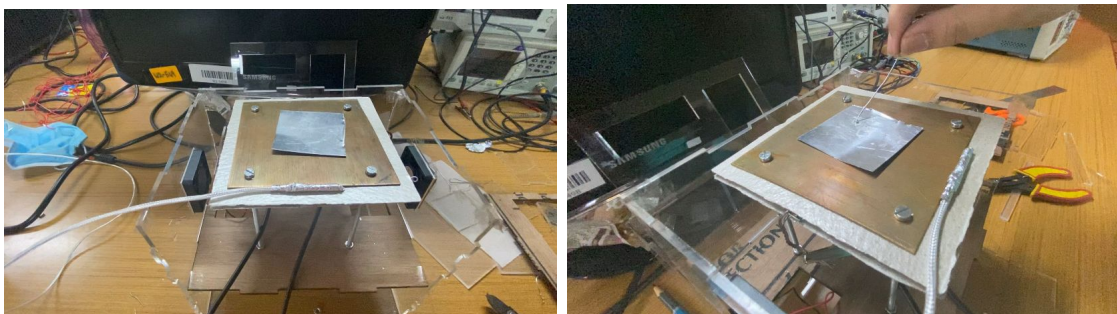
Figure 35: The final heating module setup(left) and melting of solder wire on it(right)
